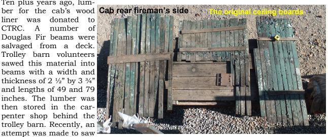
the lumber to the required thickness. It was quickly learned that the proper tools were not available and a wood shop was contracted for this work. Returned material was just slightly over the needed three-quarter inch thickness. Jerry Lane allowed the use of his planer to mill the planks down to the three-quarter inch thickness. Planks are now being sanded and prepared for the next step, milling tongue and groove edges.
