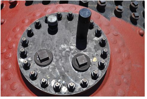
As restoration of the locomotive continues to move forward, a covered storage area is becoming more important. Again, the locomotive's boiler has begun to show affects of weather. Corrosion, which cannot be tolerated, was beginning to form upon many of the upper surfaces. Wire brushing and application of primer to all surfaces above the running boards on both sides of the locomotive is nearly complete. A coat of black paint is next.
