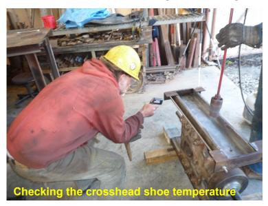
Then the babbitt and the crosshead were heated to the proper temperatures and the babbitt poured. The crosshead was then machined on the Rockford planer and the crosshead guides repositioned to match the crosshead.
