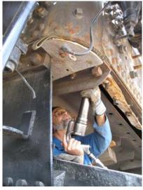
moved this operation will be completed on the locomotive. In addition the form 19's have been filed with the FRA this is for a weld repair on the boiler near the waste sheet.
