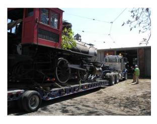
**Using** Taylor's truck for braking, Buttercup was rolled off the trailer. For the final positioning in the trolley barn, a special extended reaching fork-lift from A-Tool Shed was utilized. The special ramp constructed by John Blaine performed flawlessly as the height clearance at the barn door was near zero!
