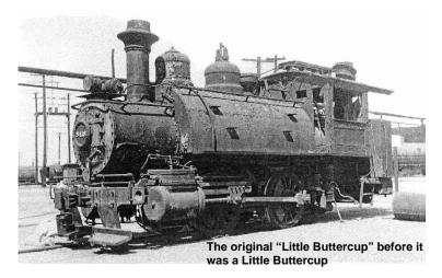
Baldwin as Santa Fe Terminal #1, for operation in San Francisco's China Basin. Afterwards, it served as the shop switcher at Needles. In 1948 the Santa Fe rebuilt the locomotive to an "old timey" appearance for historical display at the Chicago Railway Fair. The saddle tank was removed and replaced with an oversized tender. To complete the appearance, a large smokestack, headlight, and color paint scheme were added.
