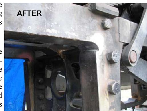
Also started this week was the chamfering of the telltale holes for all new staybolts. Chamfering of these holes is necessary to hold a sealing material that blocks soot and other debris from blocking these holes during operation. During side sheet, throat and combustion chamber repairs, close to 1000 staybolts were replaced. Each of these bolts must be chamfered.
