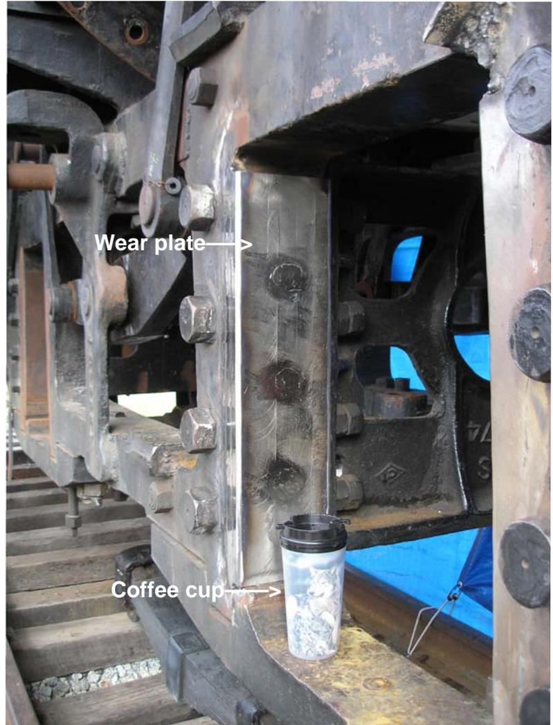
chining a new wear plate, test fitting and finally weld the new wear plate into place. In addition to the wear plate a number of defects were correct in the frame and the other wear plates as well. This process turned out to be very labor intensive. Additional the spring hangers are being machined to height.
