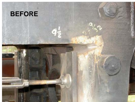
The pedestal crack was discovered during repairs to the four face plates of the number 2 driver pedestals. Each face plate's attaching welds had cracked nearly all the way around. During the weld repairs to these plates, the shoe face plate on the left side twisted
