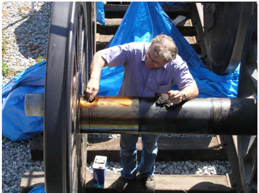
Art Randall cleaning the bearing surface
