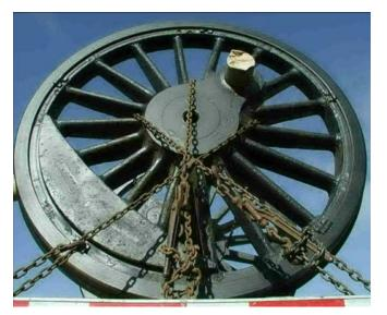
nal boxes to the Locomotive site. The drivers and journal boxes are a work of art. All the defects that were identified prior to shipment have been repaired. The pins were turned and quartered; the tires have been cut with new profiles. Journal surfaces have been refaced and burnished rolled. Like I said a real piece of
