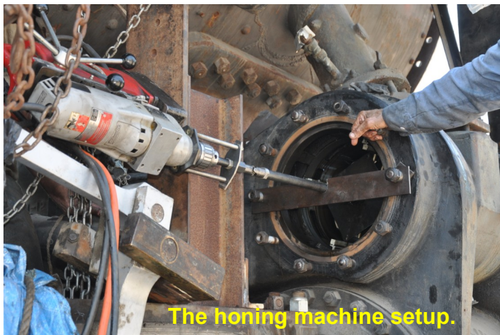
The honing machine at work
