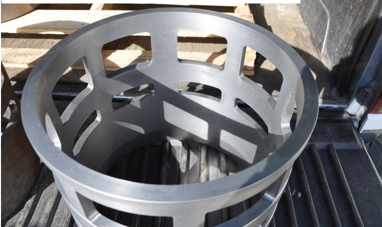
The steam distribution valve bushing
