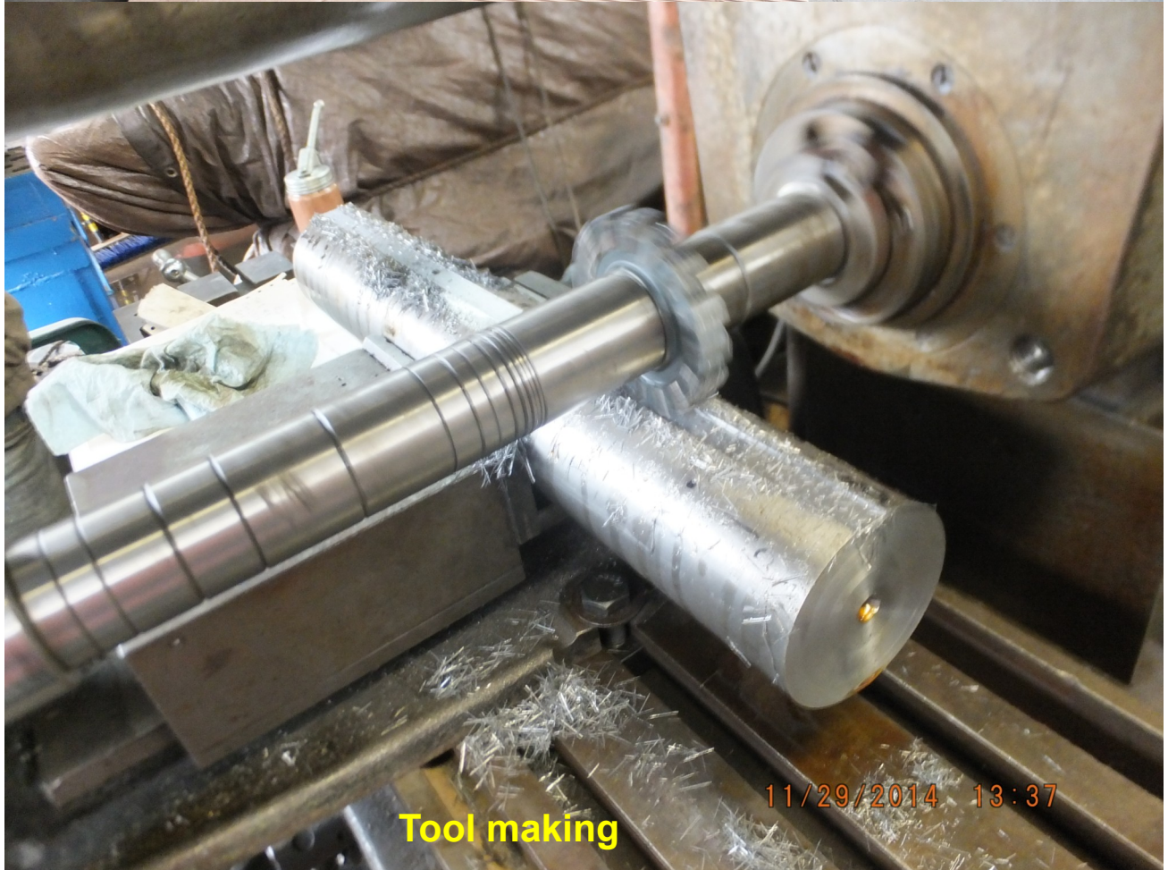
The shiny "new" power piston rod.
