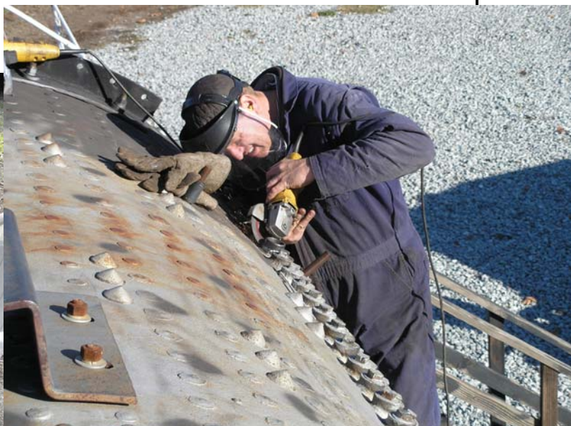
John Blaine adding sleeves to the flexible stay bolts.
