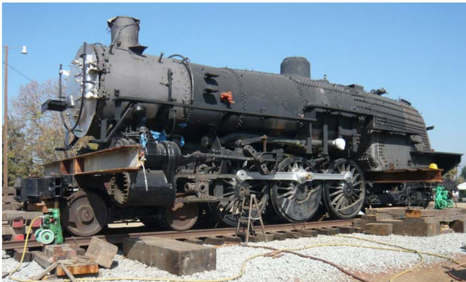
Side locomotive supports supplied by Kelly Brothers have been removed
