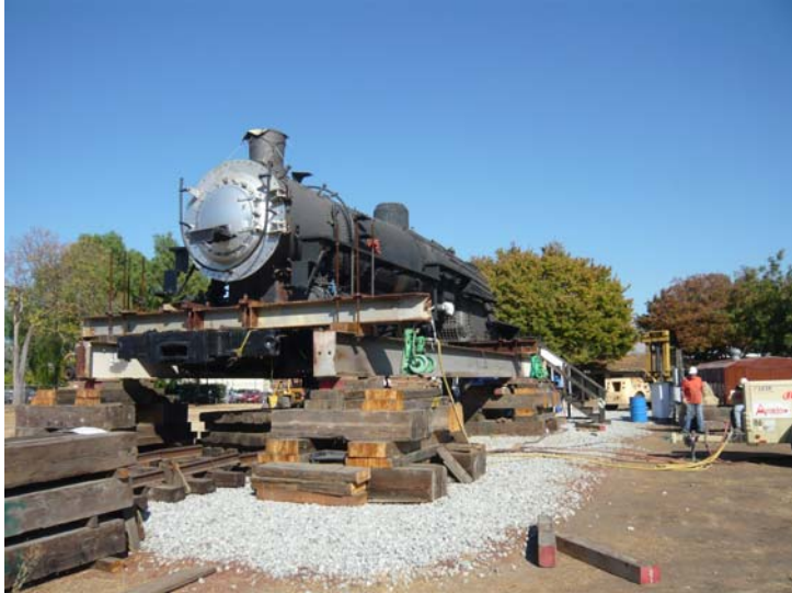
Showing the extensive cribbing required to lift the 2479
