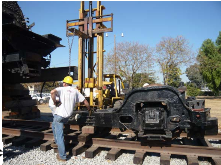
...the trailing truck needs to be moved into position
