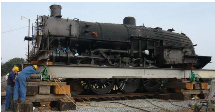
Lowering onto the wheels
