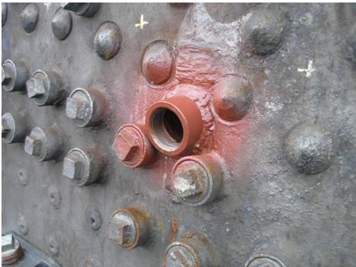
Welded fitting to back head for water column.
