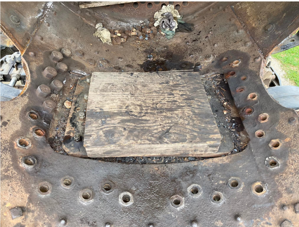
220300 Saddle bolts removal
