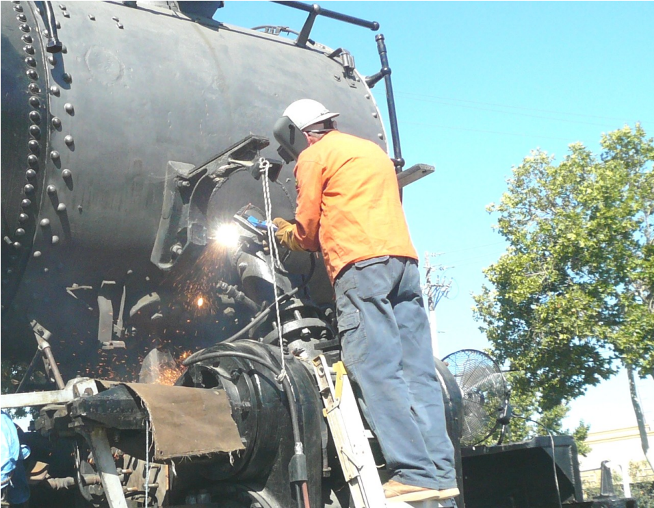
220300 Saddle bolts removal
